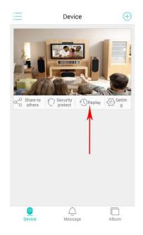
Insert a SD card into the camera and click the "Replay" to view video playback.
